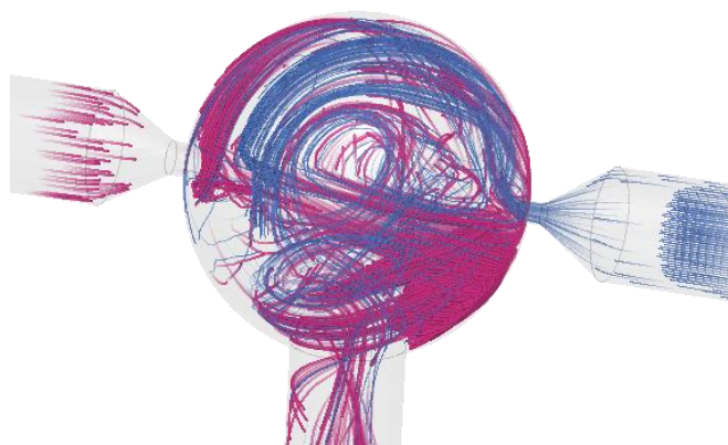
Fig. 2 Flow regime inside the FR-JET® modular mixer (TFR = 60 mL/min; Non-solvent: purple; Solvent: blue).
